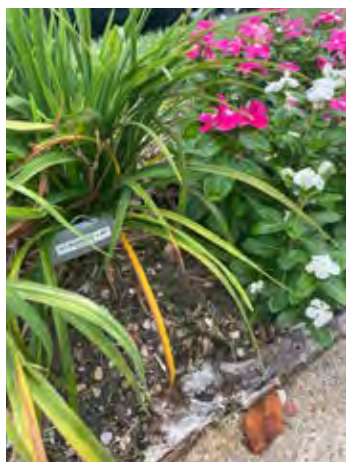
Galvanized marker with UV Inhibitor film that has stayed in the shade of the plant. Both are 4 years old, but shade makes this one look like new
